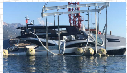
Yacht salvage using Professional Lift Bags. Photo Credit: Turismar
